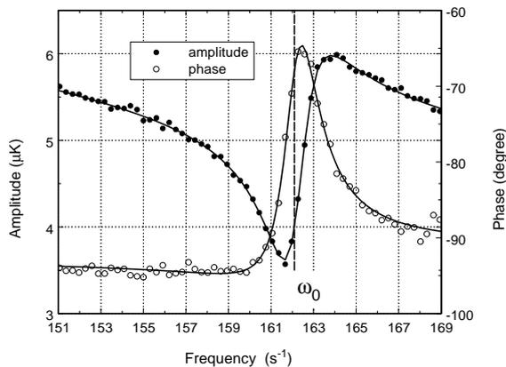
FIG. 1. Example of AFR resonance, temperature and phase shift as function of drive frequency. The solid lines are fits to Eqs. 5, 6
