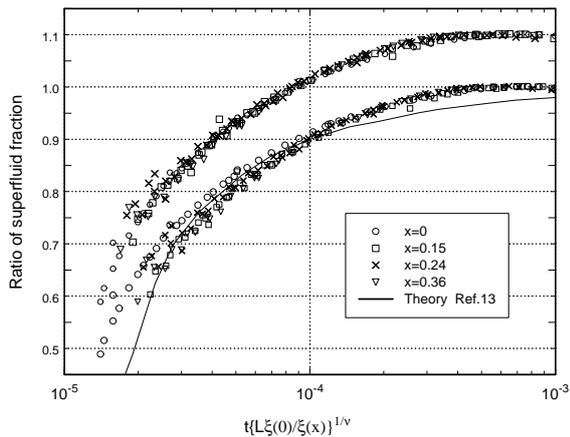
FIG. 3. Ratio of confined to bulk superfluid fractions plotted according to Eq. 7 with  $\nu=0.671$  [17]. Two values of  $L$  are used in this plot. See text. The top plot is shifted upward by 0.1 for clarity.
